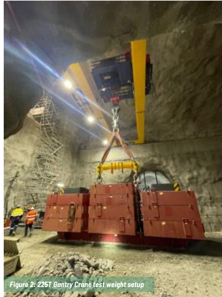
Figure 3: 225T Gantry Crane test weight commissioning process underway
